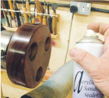
▲ Pic.13 You could probably get away without sealer but he has decided to give it a light coat of acrylic sanding sealer. Don't overdo it as it will not soak in as much on less porous timber
